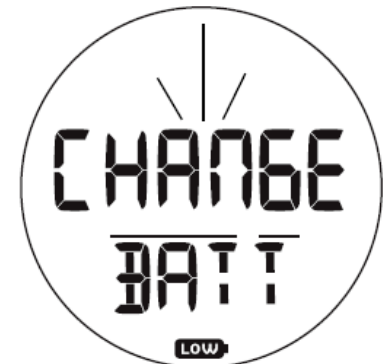
Fig. 4 - LOW BATTERY ALARM
